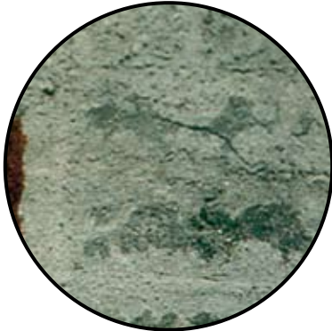
Photo 1A: Battery plate with heavy sulfation buildup.
