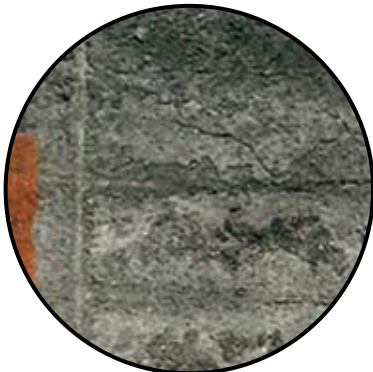
Photo 2A: Same plate 18 days later. No sulfation buildup.
